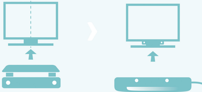
Position the mounting bracket in the middle of the screen
