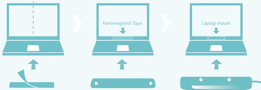
Stick the ferromagnetic tape to the middle of the screen frame
